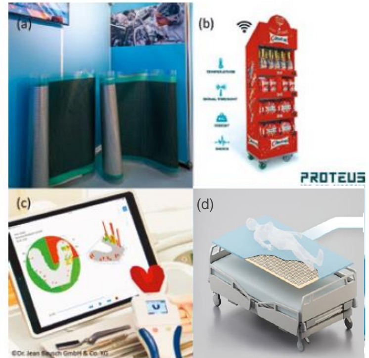
Fig. 3: The showcase of InnovationLab demonstrates the diverse applications of printed electronics with the example of printed pressure-sensor arrays. (a) Floor mat for motion detection, (b) smart shelves, (c) digital occlusion control OccluSense, by Bausch (d) smart bed
