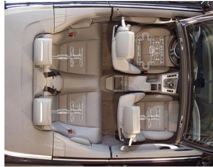
Seat occupancy detection and screen printed car seat heaters from IEE sensing
