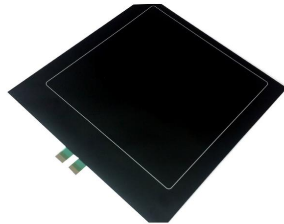
Kytronix MS9711 large area FSR matrix array sensor has 576 force sensing nodes by using 24 columns and 24 rows and is designed for true force and multi-touch detection.
